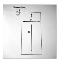
2. An additional 12 cm space in height is required for the 2<sup>nd</sup> Room adapter and duct connection.
